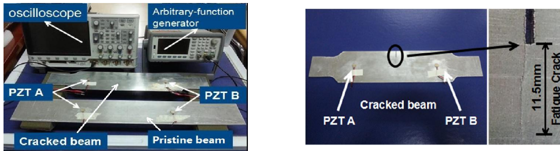
Figure 6. The experiment equipment (left) and specimens (right)
