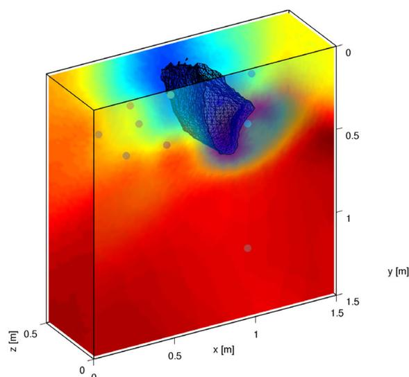
Figure 7 : Result of coda wave tomography for 20 kN load, change probability plotted color code in a semi-transparent way (red: low, blue: high). A certain level of change probability is plotted in addition as a 3D surface.
