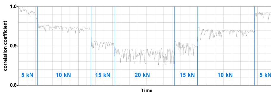
Figure 3 : Correlation coefficient change under load for a sensor pair close to the borehole
