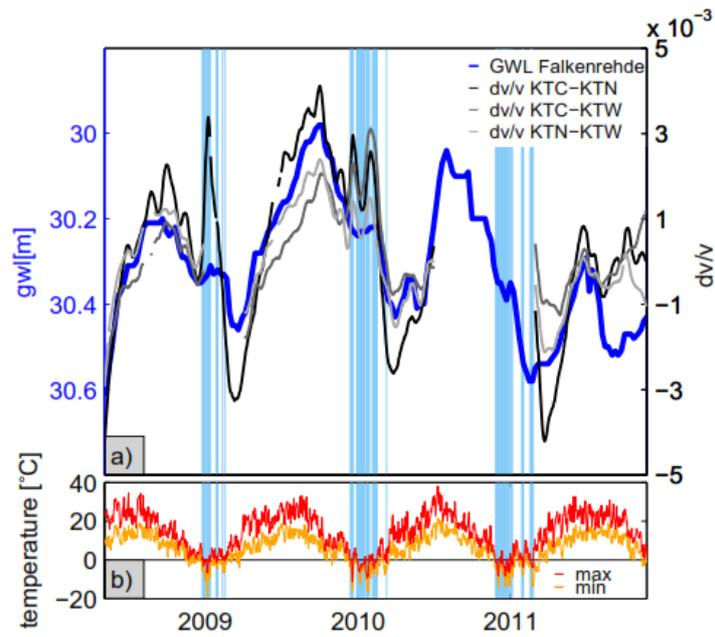
Figure 2: Velocity changes for three station pairs at the CO<sub>2</sub> storage site compared to environmental parameters. The strong correlation with the changes in groundwater level (gw, in blue, axis in m above sea level) is obvious.
