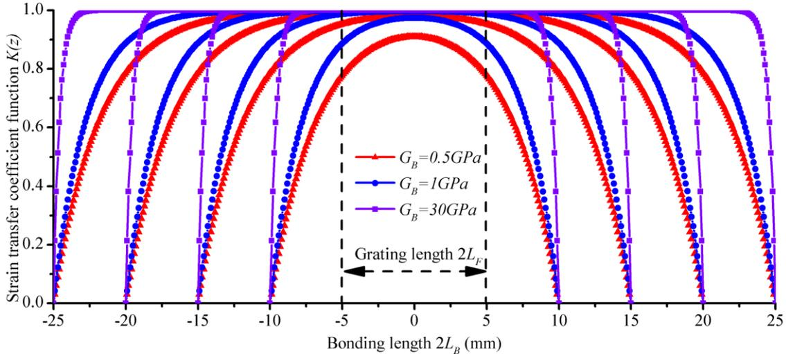
Figure 3: Function  $K(z)$  of different shear modulus  $G_B$  under different bonding length  $2L_B$ . (Parameter values set in this simulation are  $E_F=74\text{GPa}$ ,  $r_F=62.5\mu\text{m}$ ,  $h_B=0.4\text{mm}$ )
