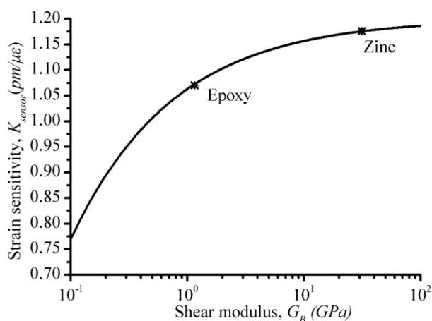
Figure 4: Relationship of the bonding material’s shear modulus to the FBG sensor’s strain sensitivity (Parameter values set in this simulation are  $L_B=20\text{mm}$ ,  $\lambda_B[1-n_{eff}^2(p_{12}-\nu(p_{11}+p_{12}))]=1.2 \text{ pm}/\mu \epsilon$ )
