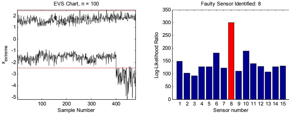
Figure 4. EVS control chart for damage detection (left) and likelihood ratio for damage localization (right).
