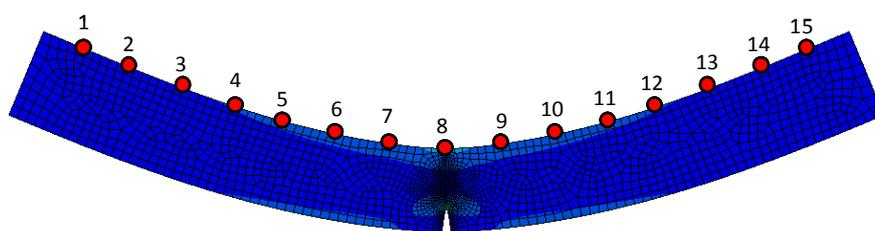
Figure 3. Monitoring of a cracked beam with 15 accelerometers.
