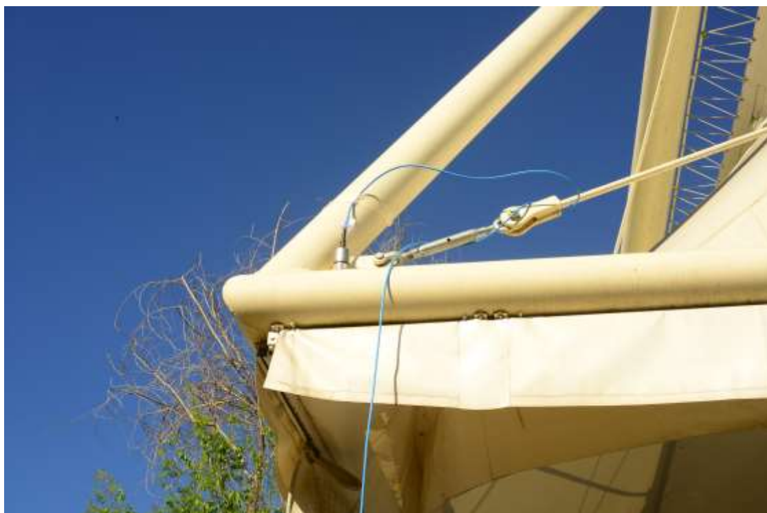
Figure 5: Sensors in field vibration test
