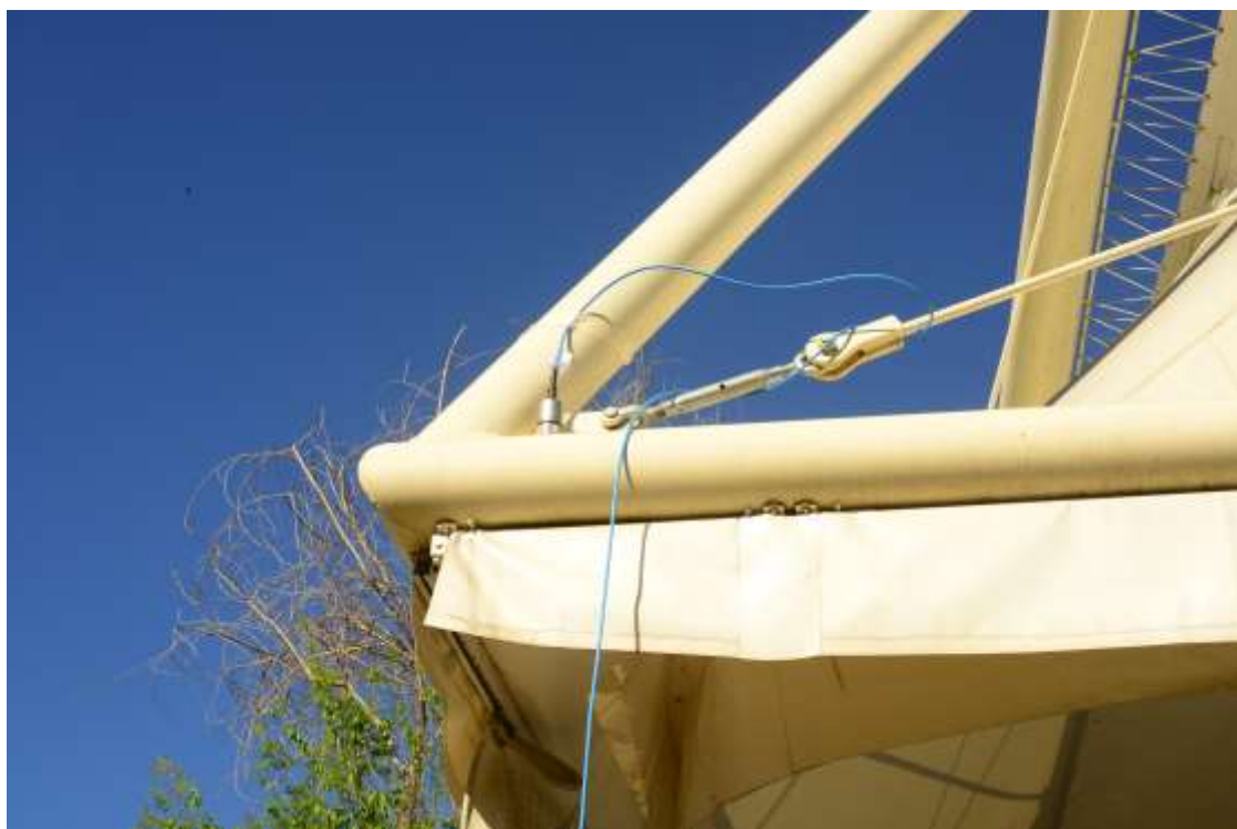
Figure 5: Sensors in field vibration test
