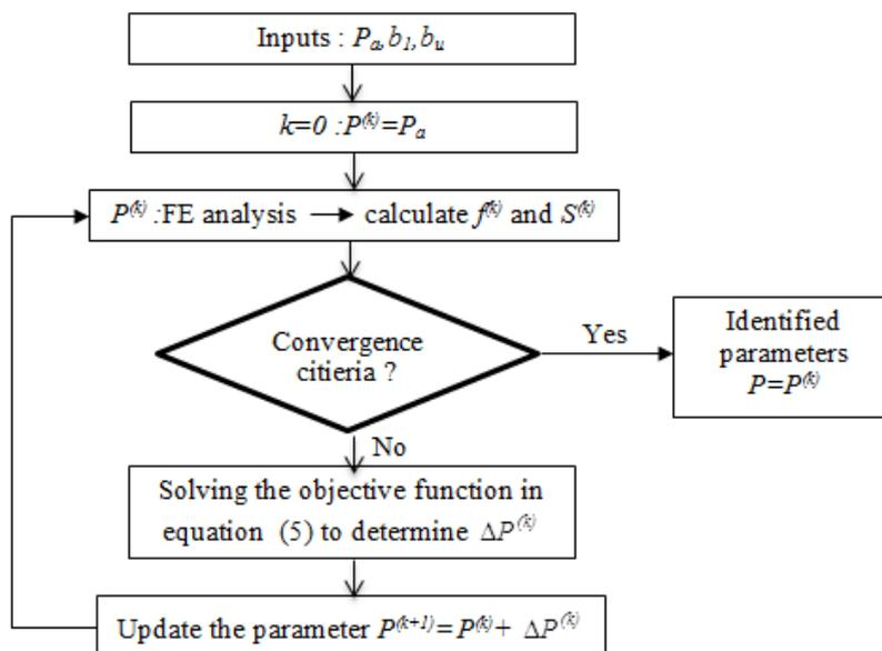
Figure 1: Sensitivity-based FE model updating procedure
