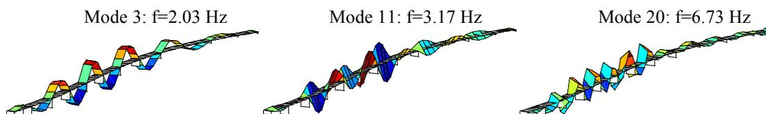
Figure 4: Selected mode shapes identified by FDD.
