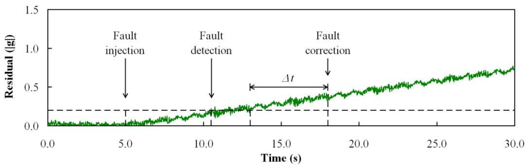
Figure 5: Residuals associated with a sensor drift
