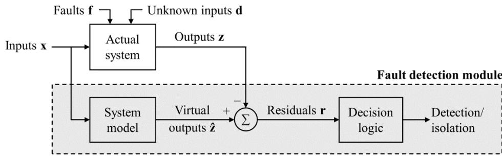
Figure 1: Conceptual structure of the embedded fault detection modules
