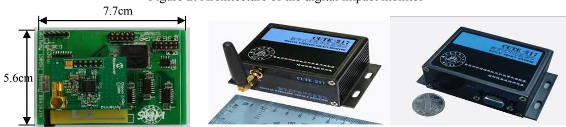
Figure 3: The miniaturized PZT-based impact monitors
