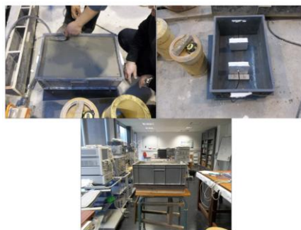
Figure 6: Experimental setup for two patch antenna embedded in concrete slab L=55cm, W=36cm, H=20cm
