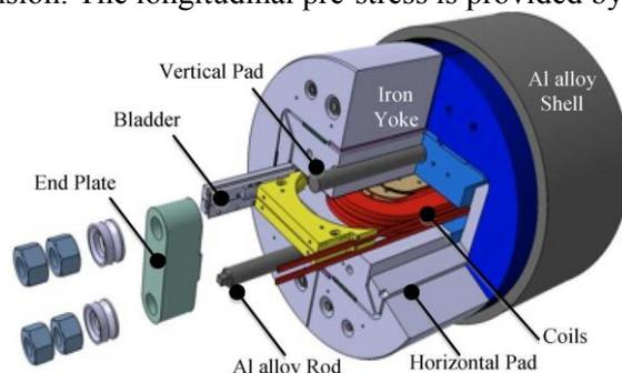
**Figure 1.** SMC structure and main magnet components
