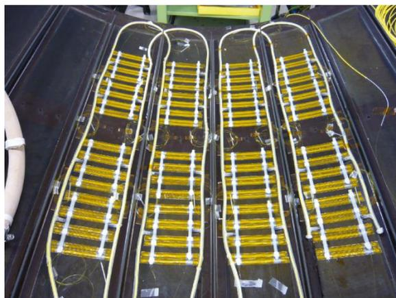
Figure 1: Hierarchical system deployed on back-surface of CFRP fuselage structure for impact damage detection [8]. Hierarchical system has wider monitorable area, higher robustness and better reparability compared to conventional fiber-optic-based systems.
