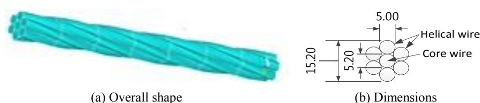
Figure 1: Structure of the considered 7-wire strand
