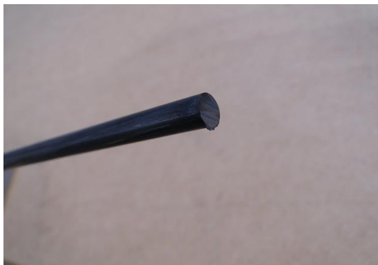
(a) Conventional steel core wire
