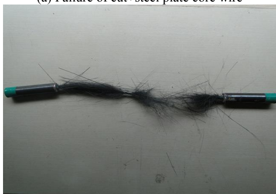
(c) Failure of pultruded core wire
