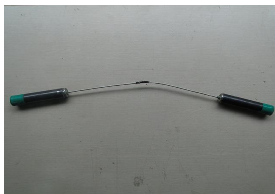
(b) Failure of braidtruded core wire
