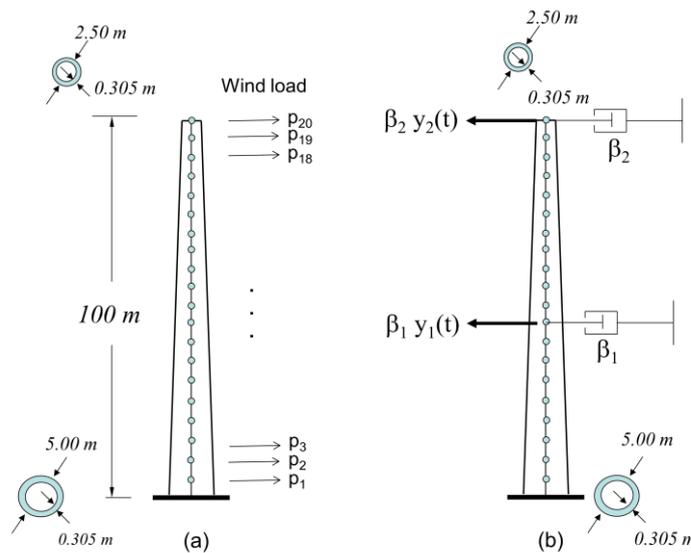
Fig.3. (a) Dimensions, discretization and loads (b) FEM-estimator
