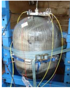
Figure 9: Composites Aquitaine™ pressure vessel burst test facility
