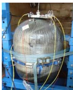
Figure 9: Composites Aquitaine™ pressure vessel burst test facility
