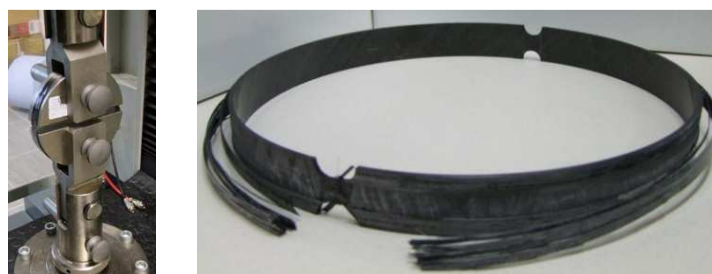
Figure 3: Experimental set-up (left) and NOL ring after failure (right)
