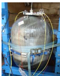
Figure 9: Composites Aquitaine™ pressure vessel burst test facility
