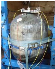
Figure 9: Composites Aquitaine™ pressure vessel burst test facility
