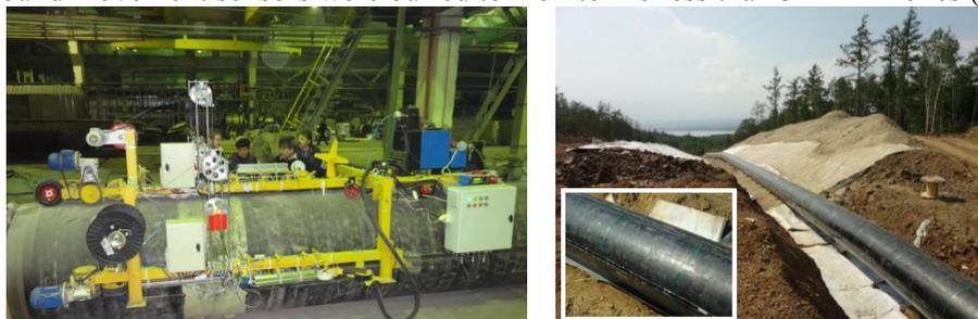
Figure 3: a) Automated machine for simultaneous integration of 3 sensors on a pipeline and b) example of field installation of 3D deformation monitoring.
