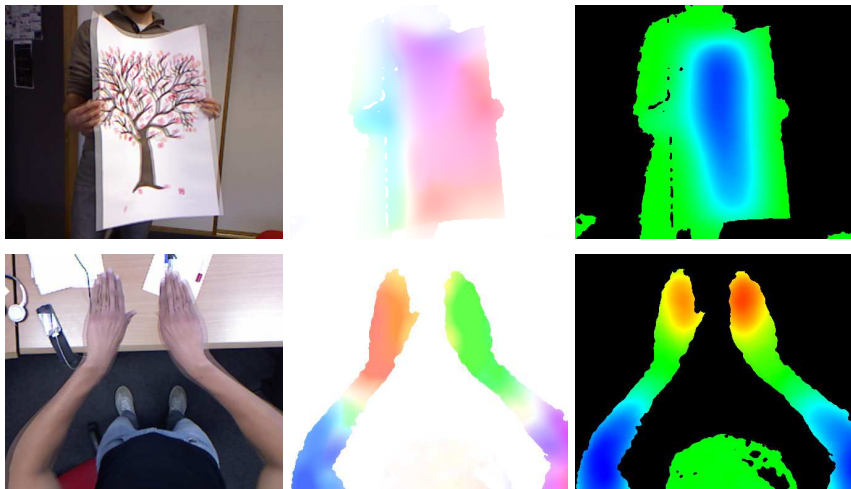
Fig. 1. Scene flow estimation with a fixed camera. a) Left : Input images. b) Middle : Optical flow c) Right : Z-component of the scene flow.
