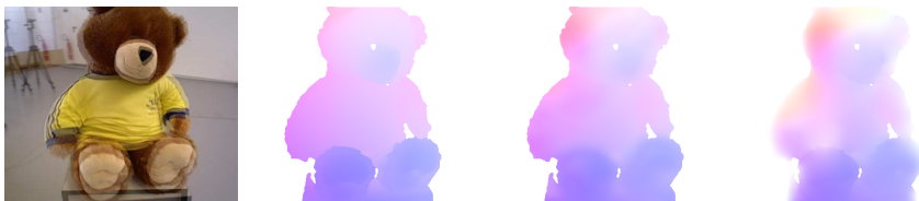
Fig. 2. Camera motion. From left to the right : a) Input images. b) Optical flow of the rigid motion estimation. c) Optical flow using the proposed method. d) Optical flow by the scene flow method [13]. Results of the proposed method are clearly more accurate than those of [13].
