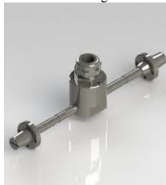
Figure 3: A vibrating wire gauge
