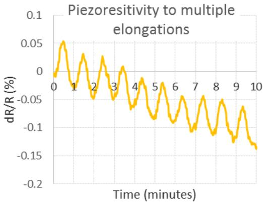
Figure 8 Response to multiple and repetitive loading cycles
