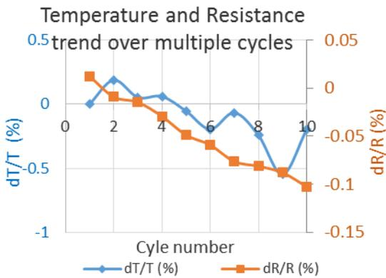
Figure 10 Average change of resistance and temperature per cycle. The average of the first cycle is taken as a reference value from which the variation  $dT$  is calculated.
