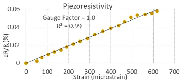
**Figure 6: Piezoresistive behaviour of CNT strain sensor**
