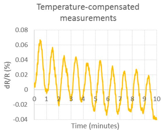
Figure 13 Temperature-compensated piezoresistivity measurement over multiple loading cycles.
