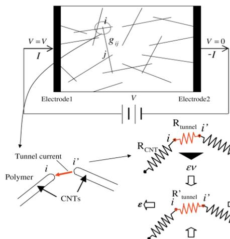
**Figure 2** Electrical model of a CNT network [13]
