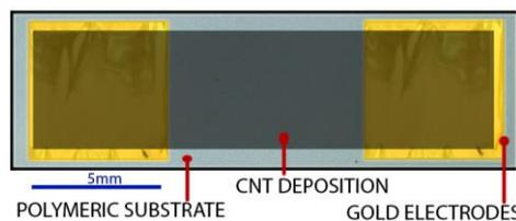
**Figure 3** Layout of the CNT strain sensor
