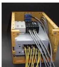
Figure 2: Onboard SHM-System for the aircraft PA200 Tornado
