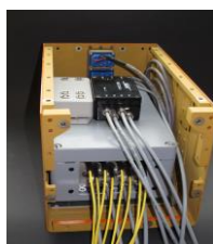
Figure 2: Onboard SHM-System for the aircraft PA200 Tornado
