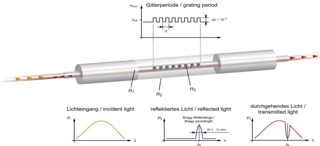
Figure 1: Caption of the figure Operation principle of a fibre Bragg grating in the optical waveguide [10]
