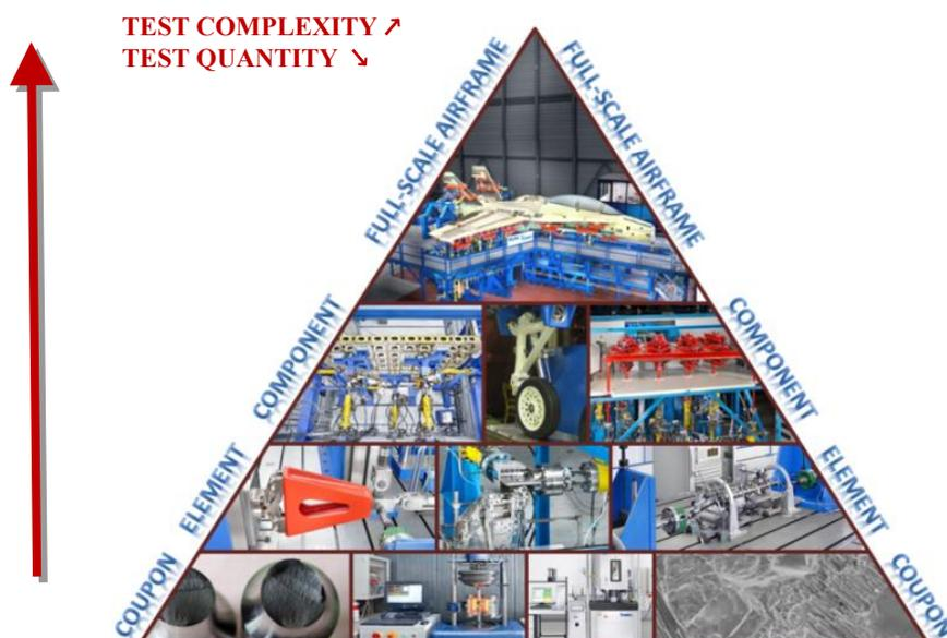
Figure 3: IABG's test pyramid for aeronautic structures
