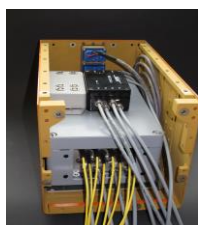
Figure 2: Onboard SHM-System for the aircraft PA200 Tornado
