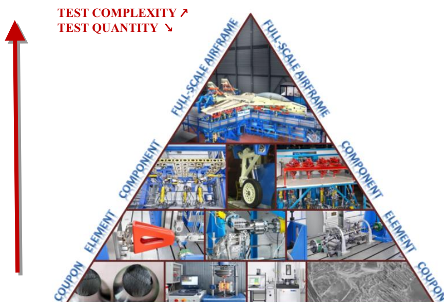
Figure 3: IABG's test pyramid for aeronautic structures
