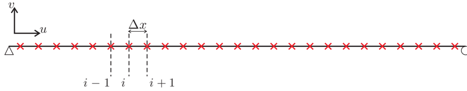
Figure 1: Regular grid of horizontal and vertical displacement sensors installed on a simply supported beam.
