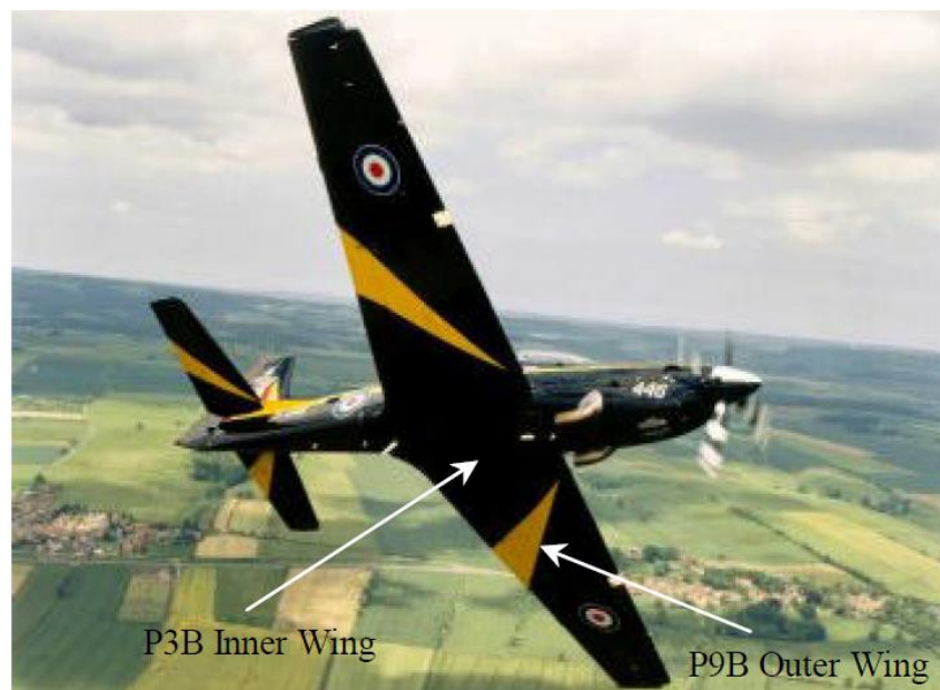
Figure 2: Short Tucano used during OLM. The locations used for monitoring strains on the port inner and outer wing are shown. [5]
