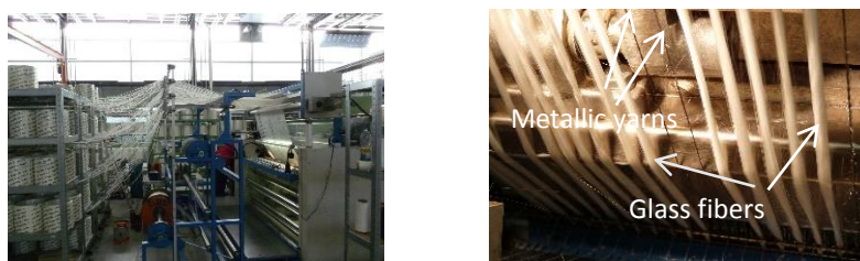
Figure1: Conductive thread insertion into warp knit.
