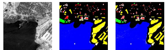
Figure 2: ((a) to (c)) Panchromatic image of Port au Prince (Pléiades, © CNES) for 2011 to 2013 respectively, ((d) to (f)) monotemporal classification maps for 2011 to 2013 respectively, (g) Classification map for 2012, obtained through the proposed cascade method using images acquired in 2011 and 2012, (h) Classification map for 2013, obtained through the proposed cascade method using all multispectral and panchromatic images.
