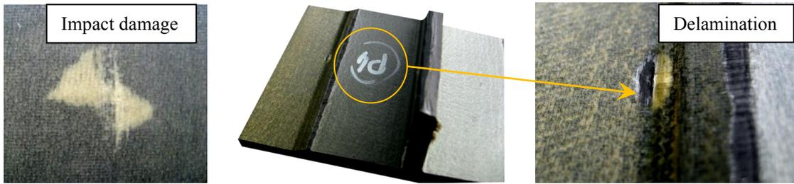
Figure 2: Imitation of FRP defects in service
