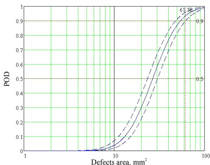
Figure 4: POD curve for CFRP service defects
