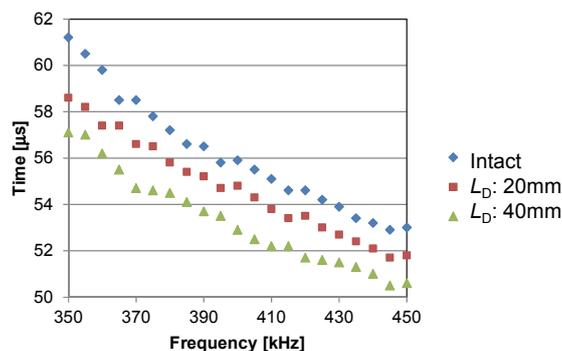
Figure 14 Maximum points extracted from the CWT results of the received  $A_1$  mode in FEA
