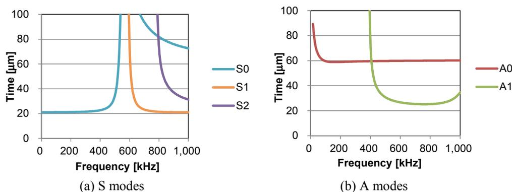
Figure 6: Theoretical dispersion curves of propagation time
