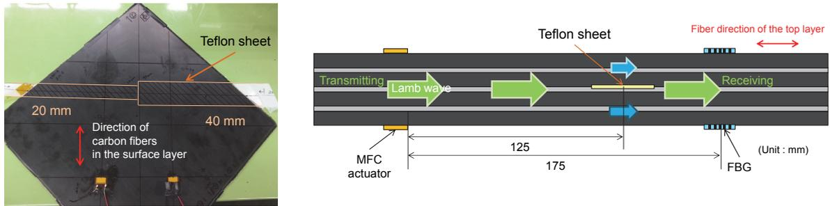
(a) Picture of the specimen (b) Cross-section of the MFL with an artificial delamination
