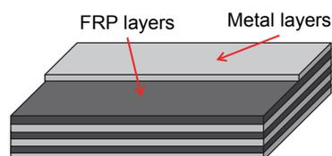
Figure 1: Schematic of FML
