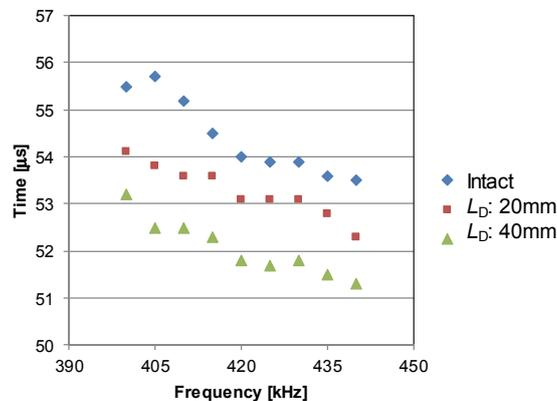
Figure 13 Maximum points extracted from the CWT results of the received  $A_1$  mode in experiments
