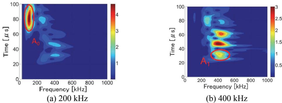
Figure 8: CWT results of A mode transmitting and receiving in the intact area
