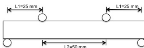
Figure 3: Schematic four-point bending setup
