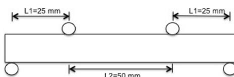
Figure 3: Schematic four-point bending setup
