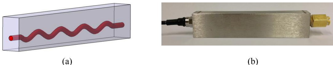
Figure 2: (a) 3D Schematic representation of feasibility test samples (b) Four-point bending feasibility test sample with installed pressure sensor
