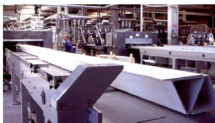
Figure 4: Pultruded profiles assembled to form a load-carrying bridge girder
