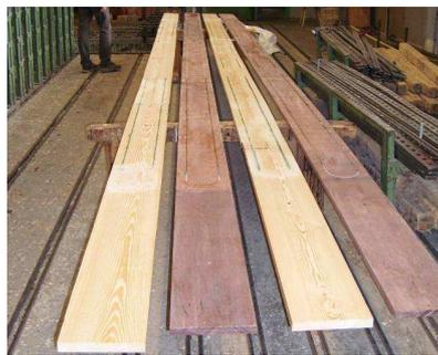
Figure 6. Application of the sensor fibres to the surface of timber lamellas before completing the glued laminated timber girder at Schaffitzel Holzindustrie GmbH in Schwäbisch Hall/Germany.
