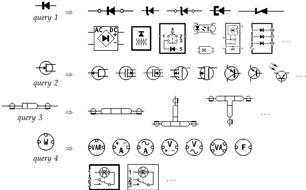
Fig. 9. Some examples of electrical symbols (Tooley & Wyatt, 2008). For every query symbol: *query 1* to *query 4*, a few relevant symbols are enlisted based on human evaluation. It consists of both linear as well as symbols in the composite form.
