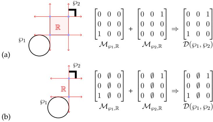
Fig. 4. A *disconnected* pair of  $\varphi_1^{\text{circle}}$  and  $\varphi_2^{\text{corner}}$  including unique reference point set  $\mathbb{R}$  and directional relations using MBR with respect to  $\mathbb{R}$ . MBR is applied for both visual primitives and combined together.
