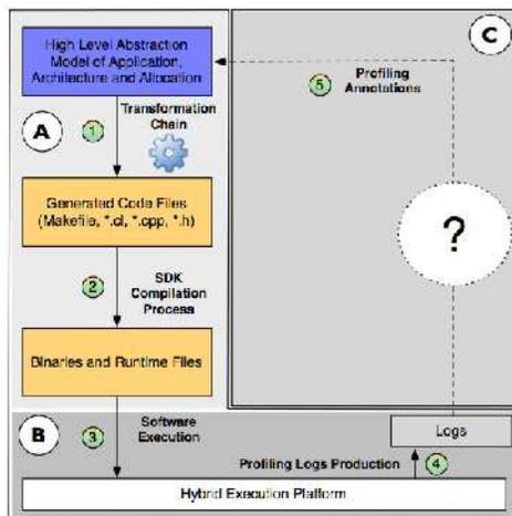
Figure 1a. Towards Integrating Profiling and MDE Compilers
