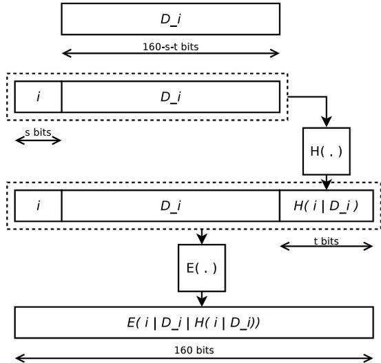
Fig. 1. Creation of the forged content identifier.
