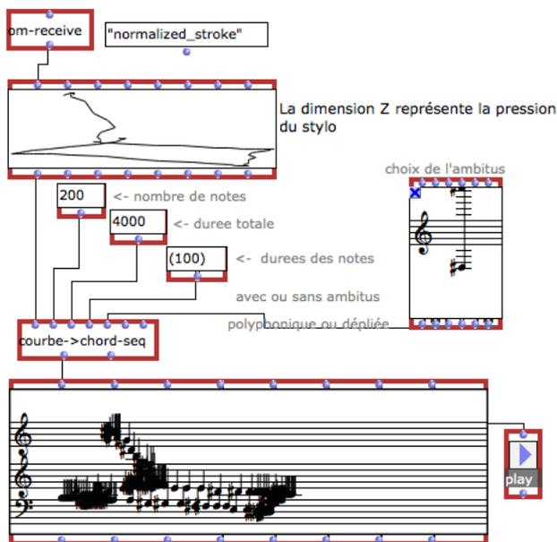
Figure 8: Converting a shape into a polyphonic sequence.
