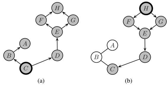
**Figure 4:** Computation of a visual program represented as a graph. (a) **Demand-driven model:** the value of box C is requested by the user and triggers the evaluation of the upstream boxes in the graph. (b) **Reactive model:** the box H has changed and propagates an update in downstream boxes whose value can be influenced by this change.
