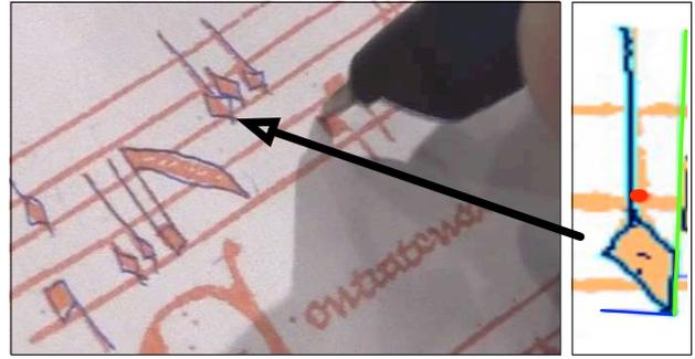
**Figure 6:** Writing on the paper interface. Left: The composer writing with the digital pen. Right: Visual feedback on the screen including the extracted shape (light-blue), its centroid (red) and main axes (blue and green).
