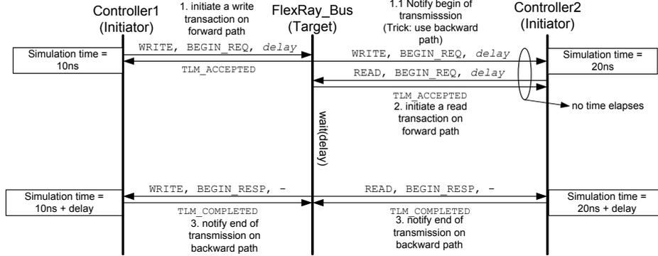
Fig. 5. Simulation of bus transmission.
