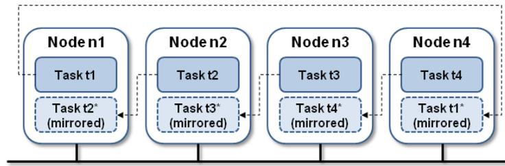
Fig. 1. Redundancy with mirrored tasks on other nodes.
