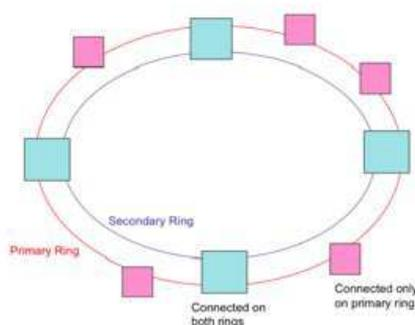
**Fig. 1.** Redundant double ring, implemented by frequency multiplex.
