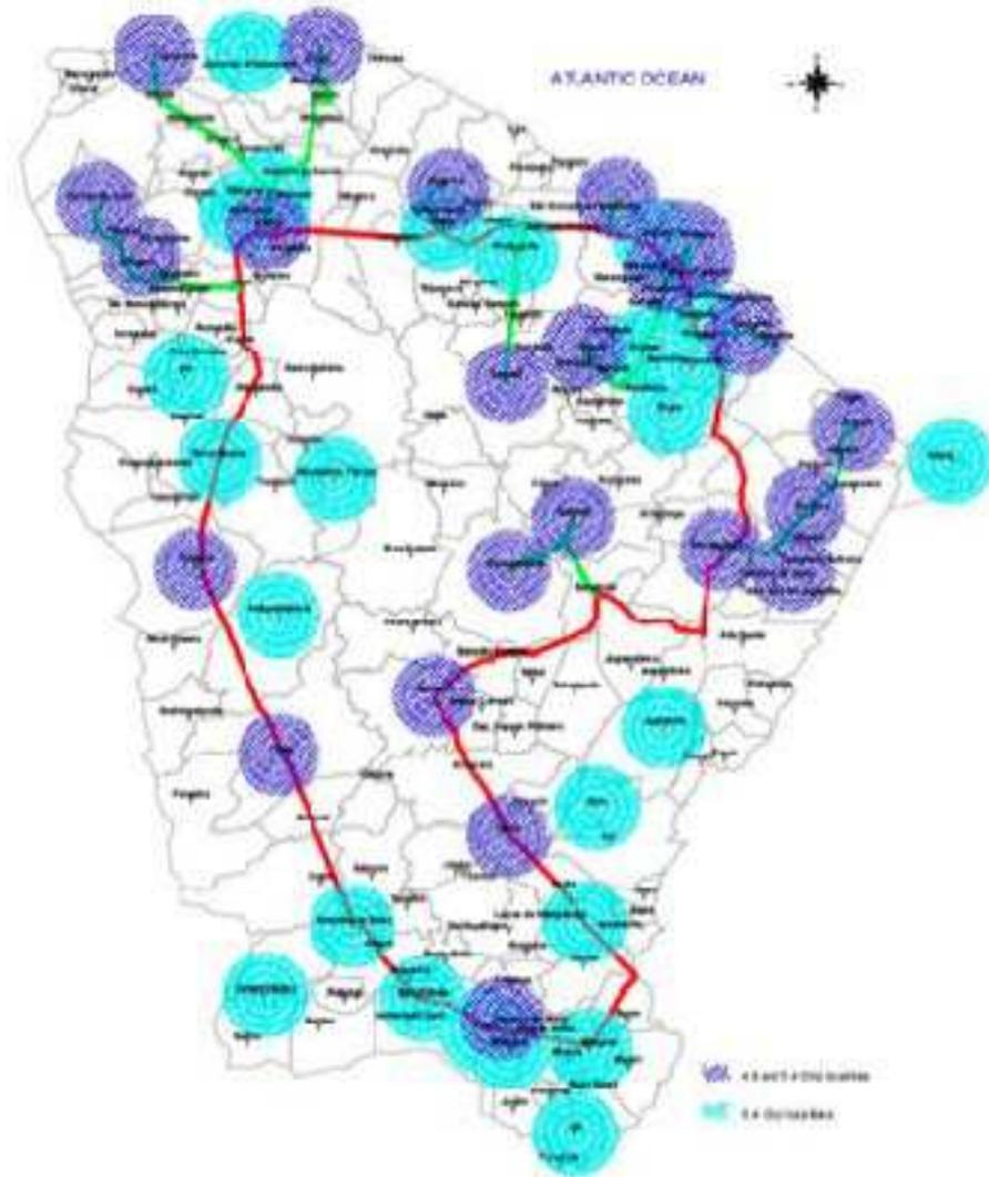
**Fig. 2.** The Digital Belt. The main redundant ring (red) the ramifications (green) and wireless base stations locations (blue).
