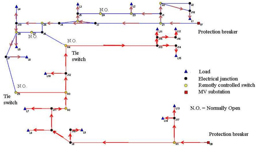
**Fig. 2.** A simplified view of MV power grid.
