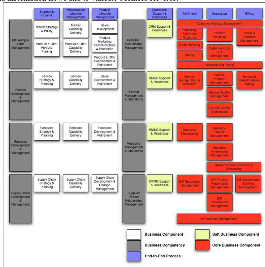
Figure 3 Business Component Map Diagram for a telecommunication enterprise
