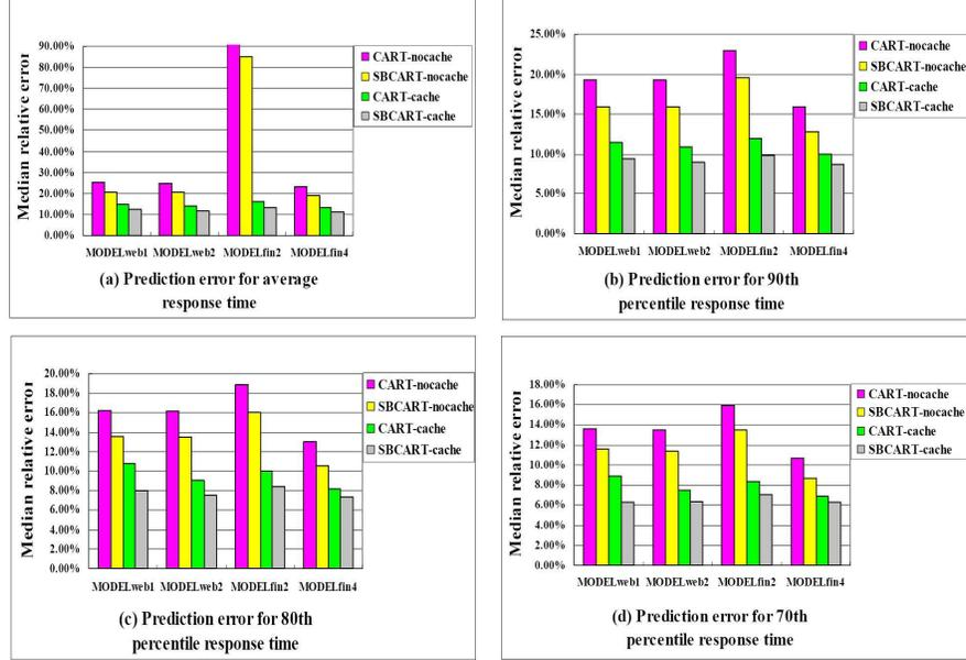
**Fig. 4.** Comparison of SBCART and CART on four traces:  $Model_{Fin2}$ ,  $Model_{Fin4}$ ,  $Model_{Web1}$ ,  $Model_{Web2}$ . CART-nocache shows that cache information (*Hit*) is not considered in feature vector and CART-cache shows that the cache information is used as a measure in feature vector.
