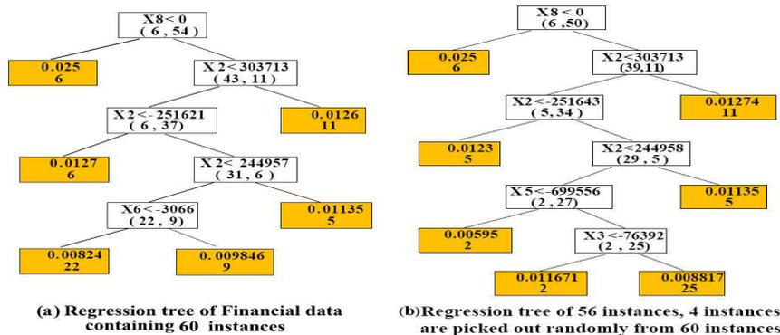
**Fig. 1.** (a) Regression tree constructed with the Financial I/O trace containing 60 instances; and (b) regression tree of 56 instances, which is produced by removing four randomly selected instances from the tree in (a). The shaded nodes represent leaf nodes containing the predicted values. The  $N_{min}$  is set to 25. More details on the Financial trace can be found in Section 3.
