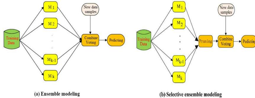
**Fig. 2.** (a) Using ensemble learning to improve the accuracy of individual basic CART models; and (b) using selective ensemble learning to improve the accuracy of a basic model. In (a), bagging or adaboost can construct a series of models  $M_1, M_2, \dots, M_k$  and then predict the unknown samples by using voting strategy; In (b), we first construct  $k$  models by bagging or adaboost, then select some representative models from  $k$  models, and use voting strategy to predict new samples.
