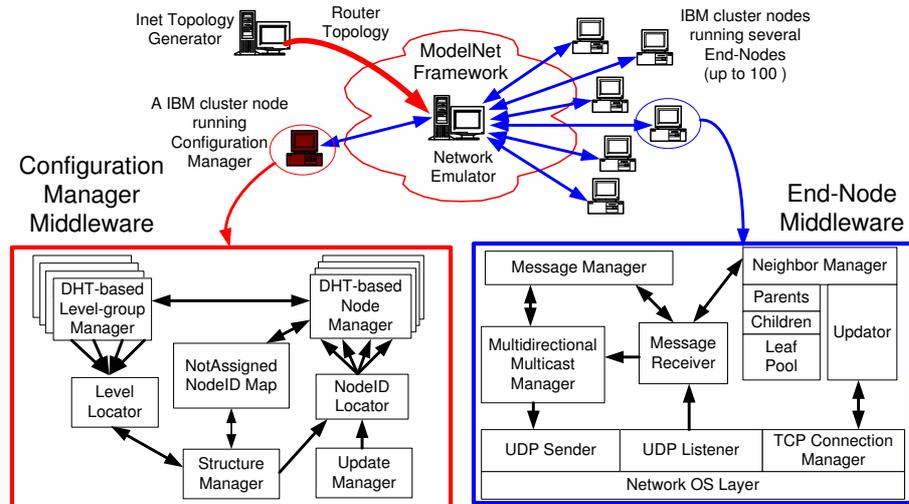
Fig. 7. FaReCast System Architecture Implemented on a ModelNet Cluster
