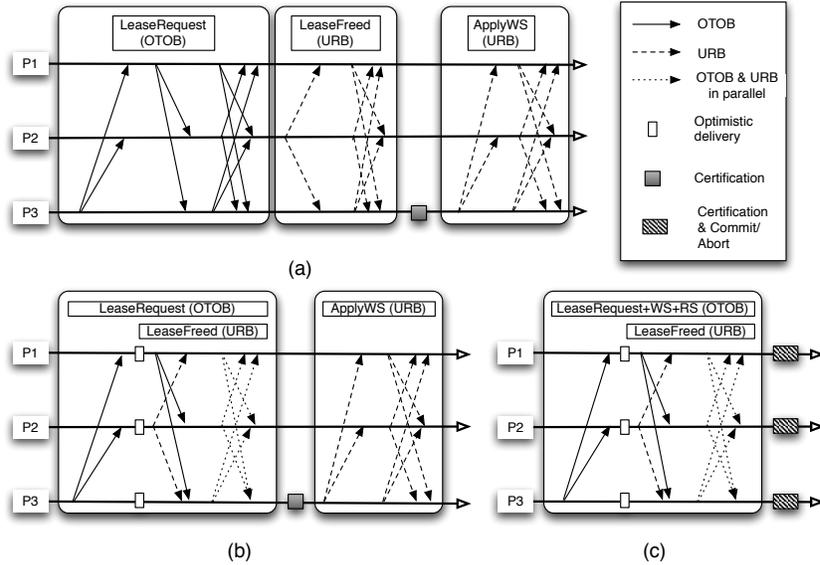
**Fig. 2.** Message pattern for (a) the baseline ALC protocol, (b) the optimization exploiting optimistic deliveries to free the leases, and (c) the optimization that piggybacks the readset and writeset on the `LeaseRequest` message ( $P3$  requesting a lease owned by  $P2$ ).
