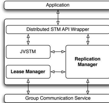
**Fig. 1.** Middleware architecture of an ALC replica.
