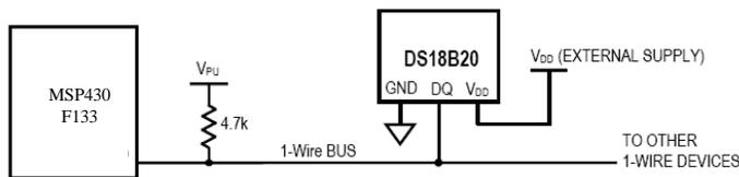
Fig.3: The interface circuit between 18B20 and MCU
