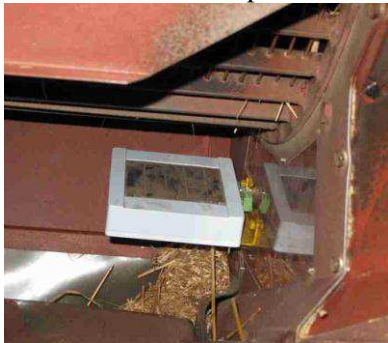
Fig.8: sensor's installation position
