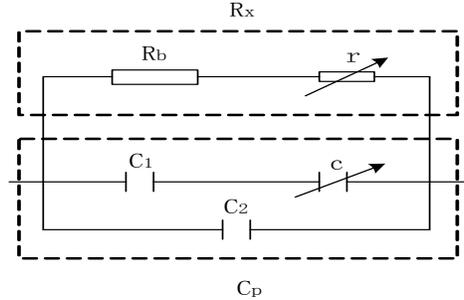
Fig.3 parallel coupling model of resistor and capacitor
