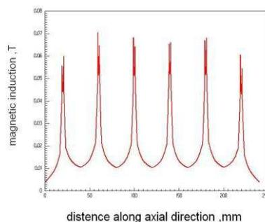
Figure 7. the curve of magnetic induction intensity in the order of NN along the axial direction
