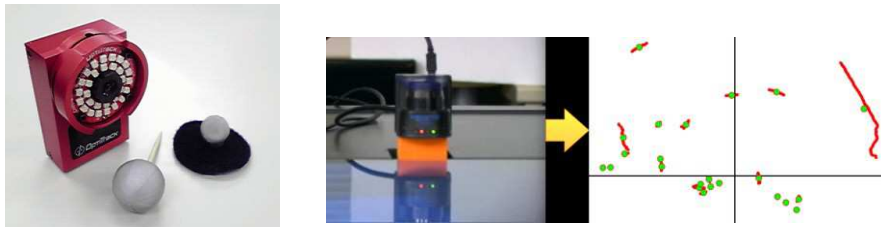
Fig. 1. An infrared camera and markers(left) and data detected by a near-infrared radar(right).
