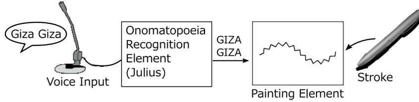
Fig. 2. System architecture
