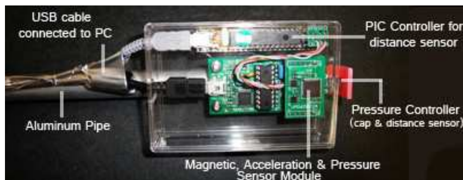
Fig. 3. VBS device structure
