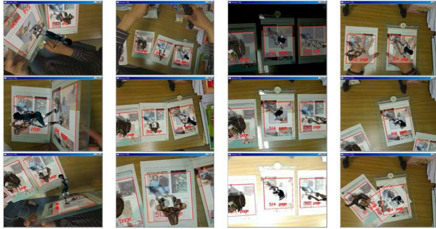
Fig. 7. Tracking in situations with dramatic viewpoint variation (1st column), scale variations (2nd column), illumination variations (3rd column), and partial occlusions (4th column)
