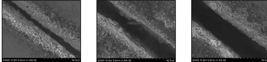
**Fig. 5.** SEM Images of Channels Made in Steel Through LIP-MM Process with 1, 5 and 10 Passes, 10 kHz Pulse Repetition Rate, Peak Power Density Level Corresponding to 70% Plasma Occurrence Probability and Laser Beam Traverse Speed of 100  $\mu\text{m/s}$
