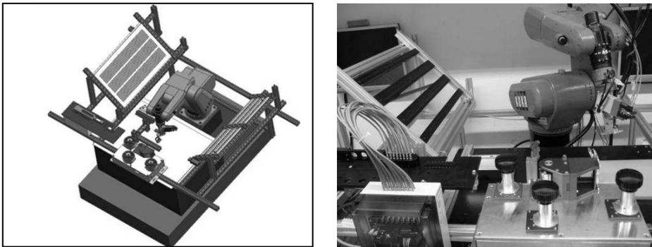
**Fig. 2.** The robotic cell includes an articulated robot (middle), two supply systems for chips and scaffolds (left and right of the robot), a feeding system for adhesive gaskets (front) and a sealing test module (front left).
