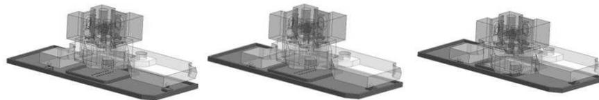
**Fig. 7.** Assembling sequence for chip and scaffold: (1) the robot gripper gets close to the scaffold, (2) the scaffold is floating on an air cushion (3) the gripper is actuated linearly in order to bond chip to scaffold
