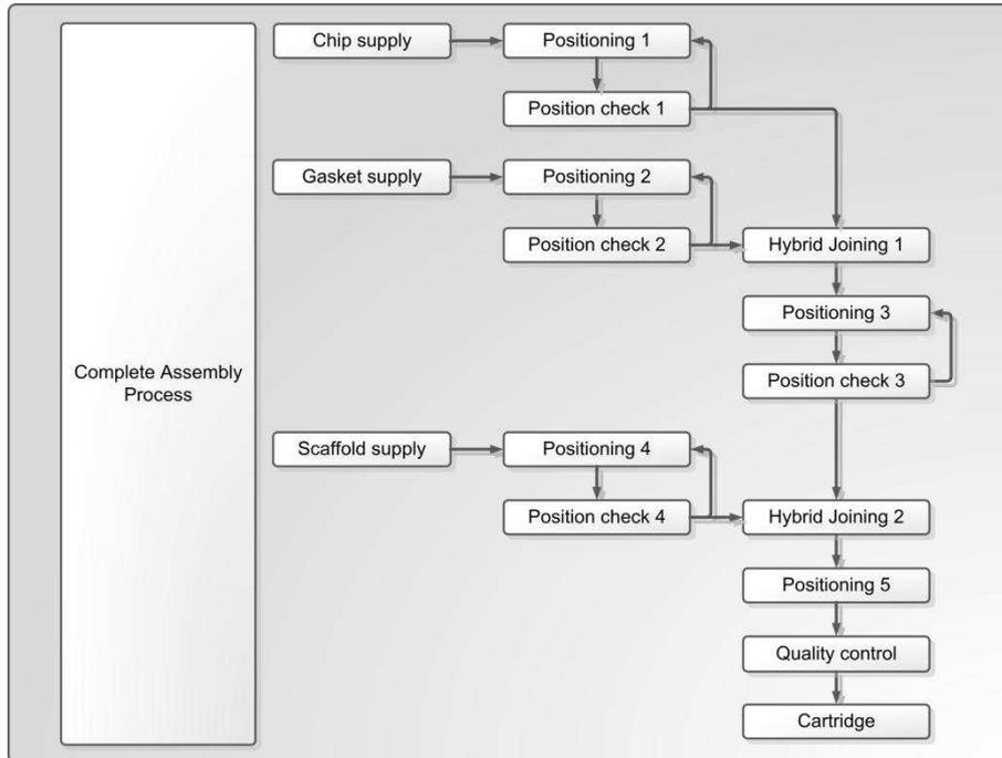
**Fig. 3.** Description of the assembly process: Exact component position is controlled before each hybrid bonding step.
