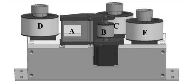
**Fig. 5.** The tape feeding system supplies adhesive gaskets automatically. Gaskets are provided on foil rolls and are covered by protection foils. Before hybrid bonding, one gasket is moved to the joining area while the protection foil is removed.
